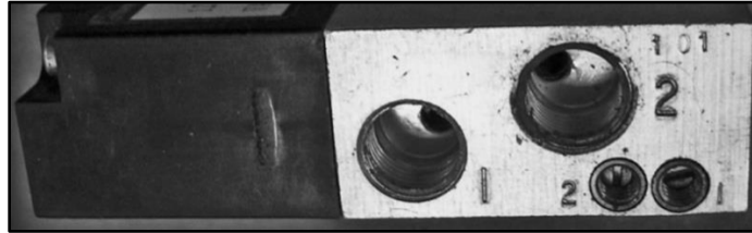
Figure 3-6 Ports Labeled 1 and 2 on Reverse Side of Solenoid Valve
