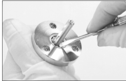
Figure 5-43 Removing the Retaining Ring that Retains the Drive Shaft
