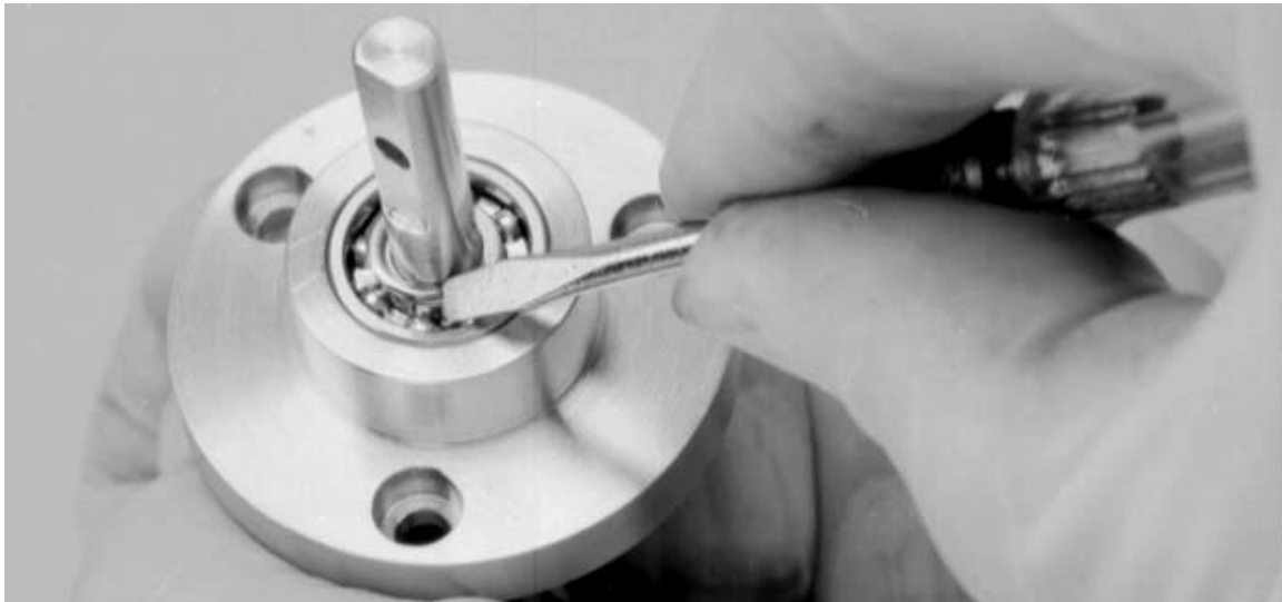
Figure 5-25. Removing the retaining ring that holds the parts of the drive shaft assembly in place
