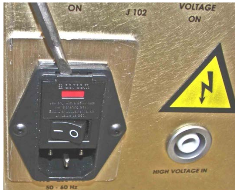
Figure 5-11 Prying Open the Fuse Block Cover on FPS Front Panel
