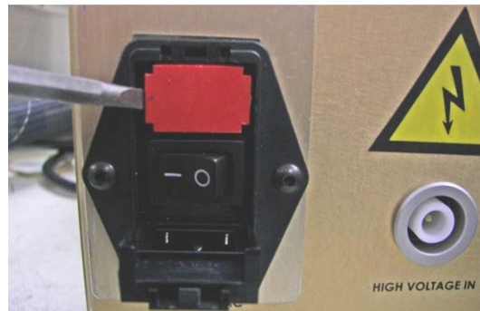
Figure 5-13 Fuse Block Removed from FPS
