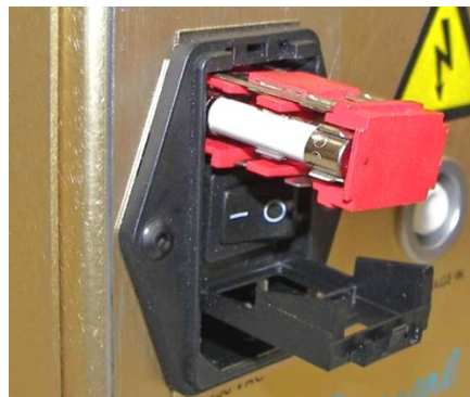
Figure 5-13 Fuse Block Removed from FPS
