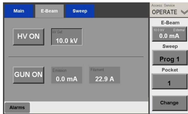
Figure 3-4 Operations&gt;E-Beam Screen, Beam On at 0.0 mA
